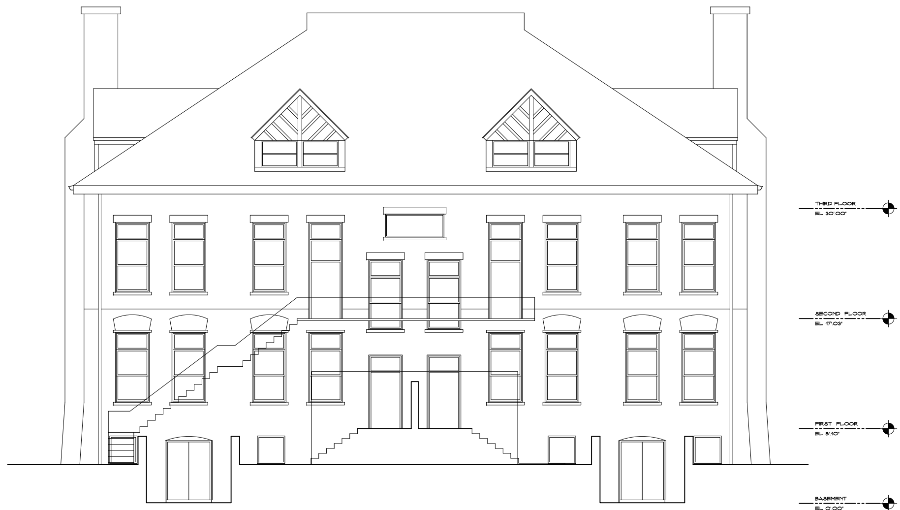
REAR ELEVATION (SOUTH) 1 A7 SCALE: 1/4" = 1'-0"
